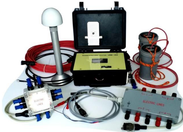
LEMI-424 system full set layout (left); LEMI-424 system in transportation case
